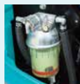
Pre fuel filter with built-in water separator
