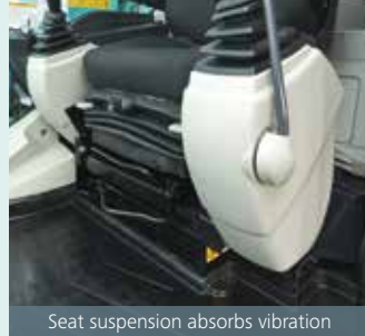
Seat suspension absorbs vibration
