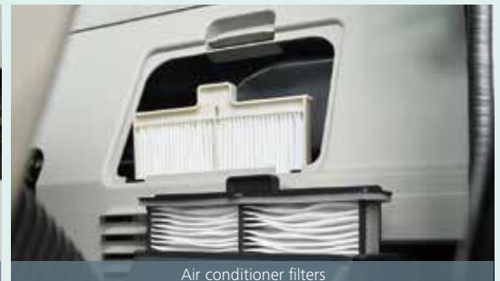
Air conditioner filters
