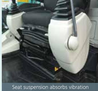
Seat suspension absorbs vibration
