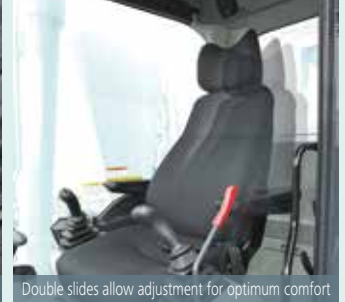
Double slides allow adjustment for optimum comfort
