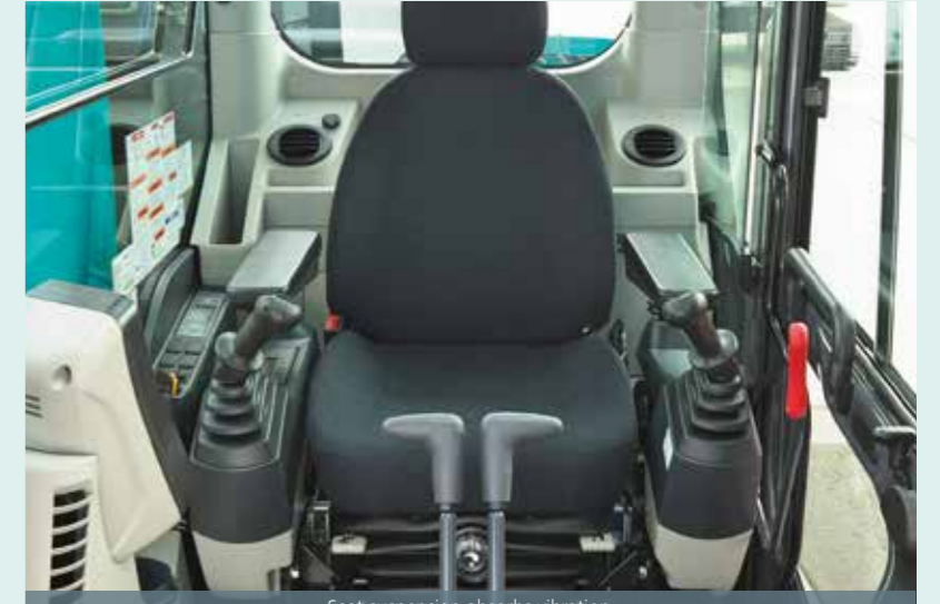
Seat suspension absorbs vibration
