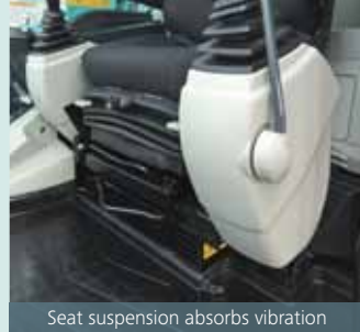
Seat suspension absorbs vibration
