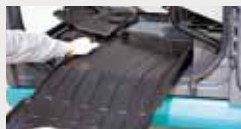
Detachable two-piece floor mat has handles for easy removal. A floor drain is located under the mat.
