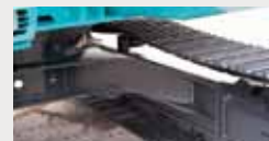
Special crawler frame design makes it easy to clean off mud.
