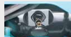
Engine quick-drain valve can be turned without tools.
