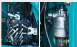
Control valve/water separator
