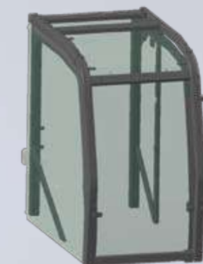
• Level 2 FOPS Guard (ISO 10262) is available as an option
