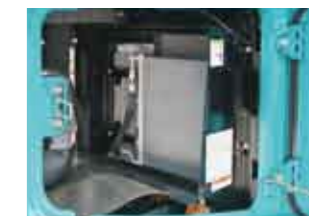
Cooling unit and air cleaner
