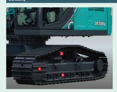
The crawlers are designed to provide unbeatable durability to take on the harshest terrain. They feature full track guides to eliminate de-tracking concerns, a reinforced guide frame built to withstand heavy impact, and large, double-support, outer flanged upper rollers unfazed by powerful vibrations.
