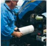
The air filter is easy to check, clean or replace with no need for tools.
