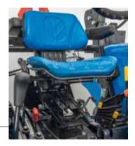
**COMFORTABLE SEAT** The mechanical suspension seat is mounted on an inclined base, to suit any size operator.
