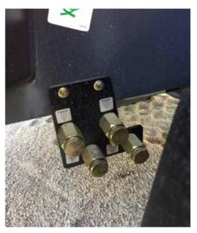
All pressure taps and sight gauges are easily accessible. Fluid drains provide environmentally friendly drainage capability and are grouped together for convenient serviceability.
