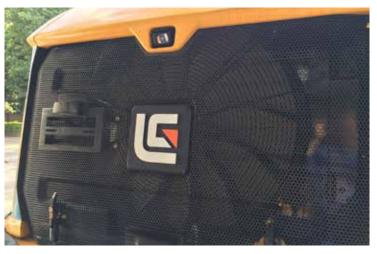
All-around visibility is supported by a rear-view camera acting as an extra eye on the jobsite.
