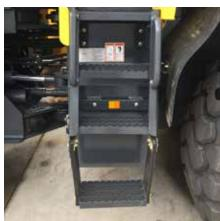
Acess to the front of the cab by the operator or service person is a new feature. The same anti-slip bars used on the egress steps are used here for maximum anti-slip protection.
