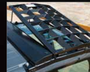
Opening TOPS guard The TOPS guard is hinged, allowing easy access to the top window for serviceability.
