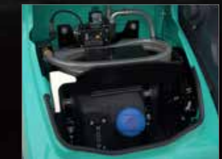
Ground level AdBlue* tank * AdBlue® is a registered trade mark of the Verband der Automobilindustrie e. V. (VDA).
