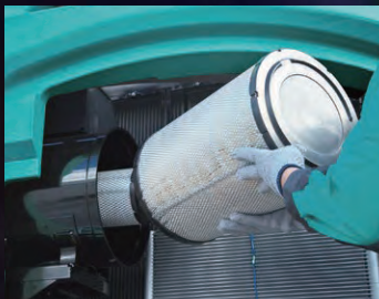
Two-stage air filter
