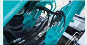
Boom & arm holding valves
