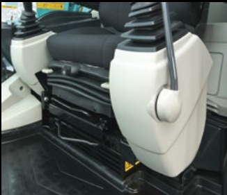
Seat suspension absorbs vibration
