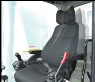
Double slides allow adjustment for optimum comfort
