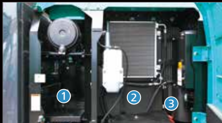
Left side (radiator and tool box space cooling system elements)
