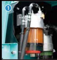
Pre-filter with integrated water separator
