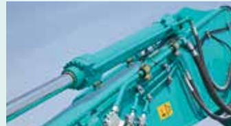
Dismantling bucket cylinder
