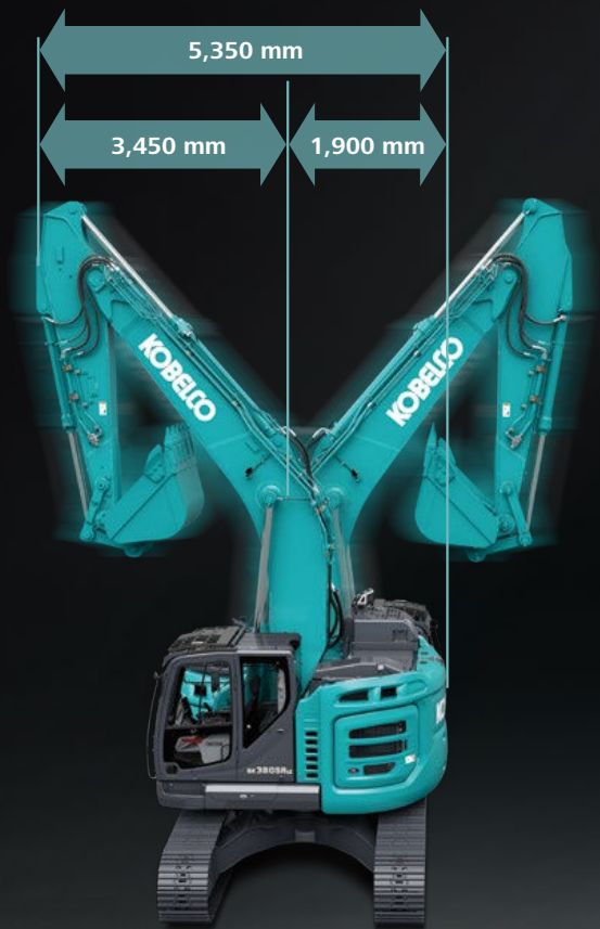
Figures above show the value for standard boom and standard arm spec.
