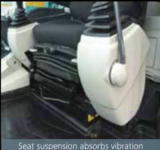
Seat suspension absorbs vibration
