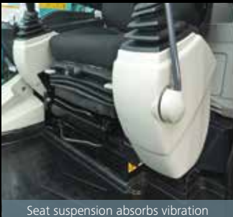
Seat suspension absorbs vibration
