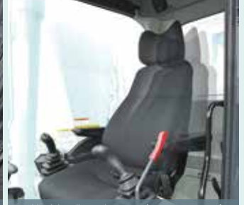
Double slides allow adjustment for optimum comfort
