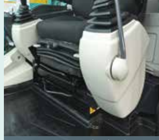
Air suspension seat absorbs vibration
