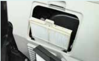
Air conditioner filter can be easily removed without tools for cleaning. One for outside air and one for inside air.
