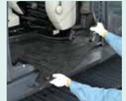
Detachable two-piece floor mat with handles for easy removal.
